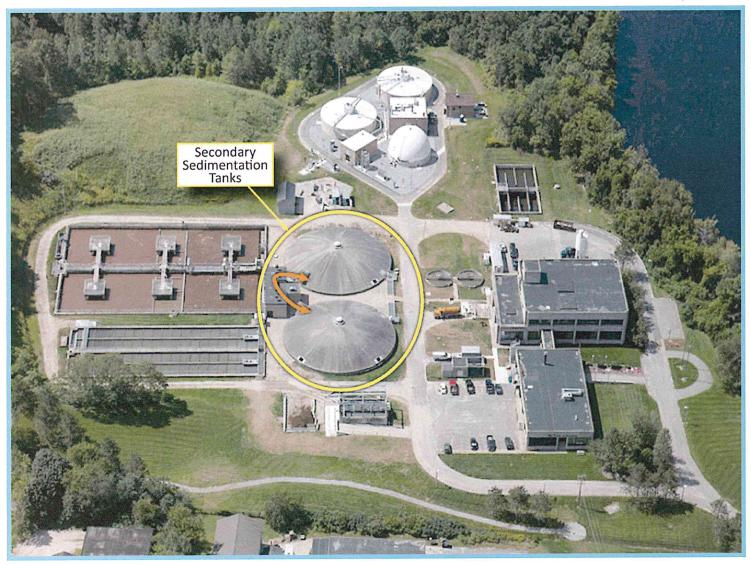
Wastewater flows to secondary clarifier tanks where the bacteria from the aeration basins are settled out of the wastewater
