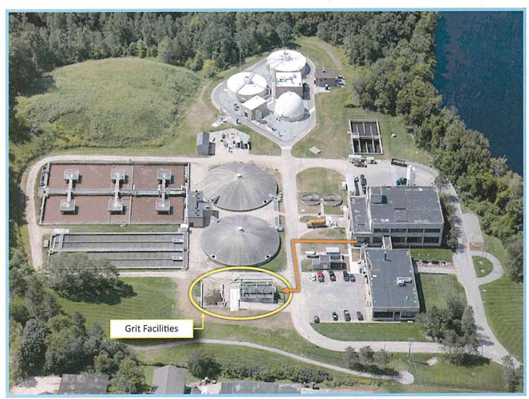
The grit facility uses air to separate heavy inorganic particles from the wastewater, leaving lighter organic particles
