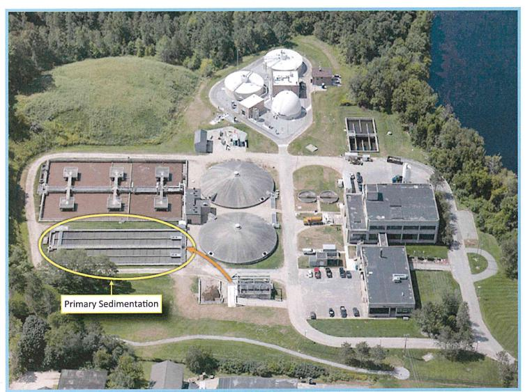
Wastewater flows to primary sedimentation tanks where more than onehalf of the solids are removed
