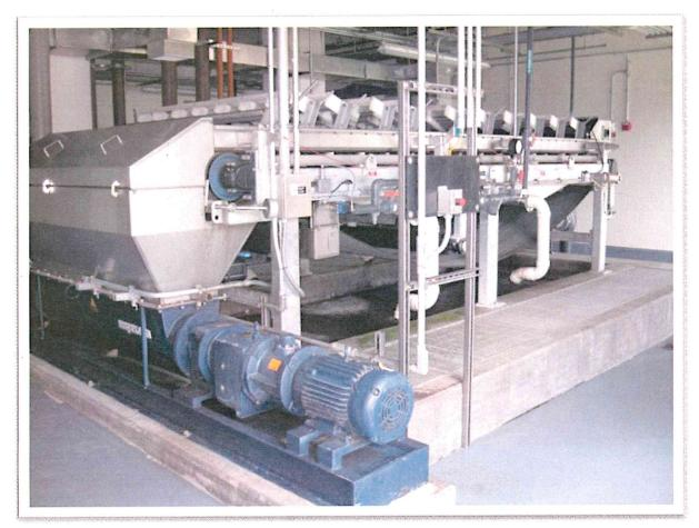
Primary and secondary sludges are treated to remove excess moisture prior to anaerobic digestion
