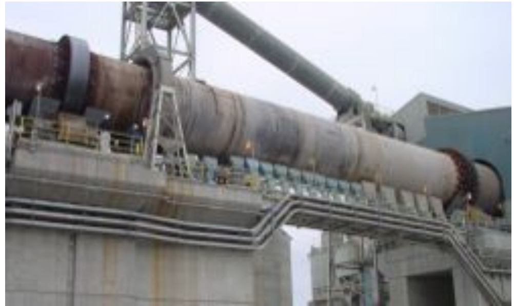
Dried biosolids are used as alternative fuel in coal-fired cement kilns.
