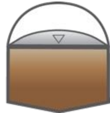
Gas Membrane Cover
