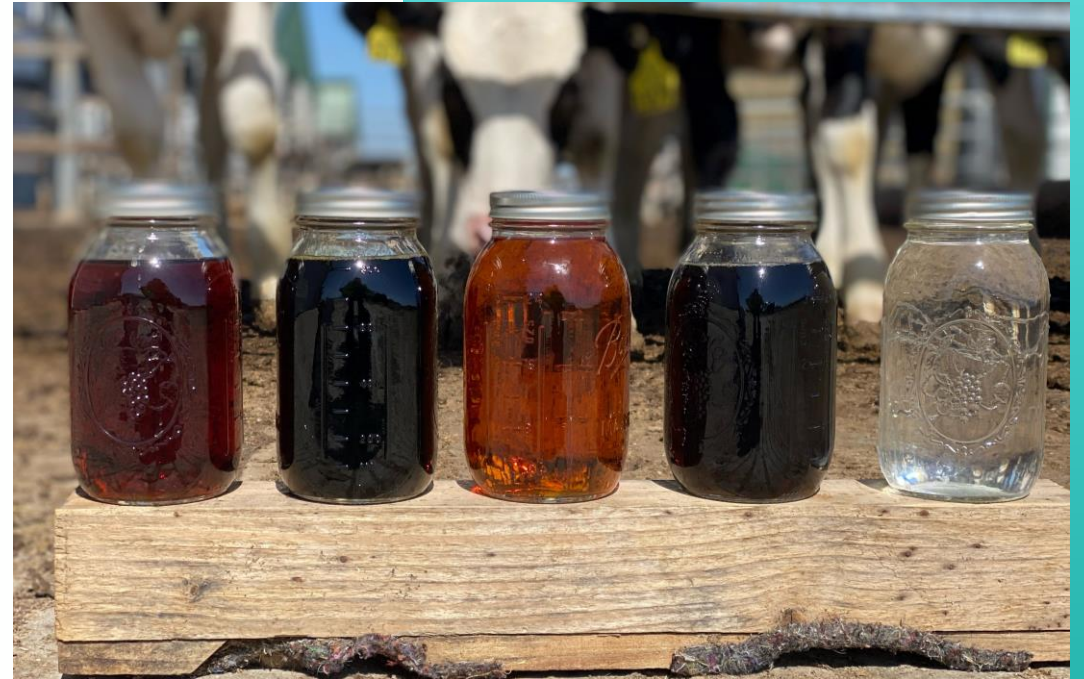
ZwitterCo SF Permeate (Center), ZwitterCo SF Concentrate (second from right), RO Permeate (far right)
