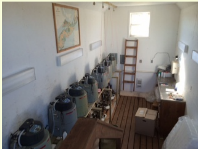
The lysimeter water collection system at the Dalhousie University (Truro) biosolids research site.
