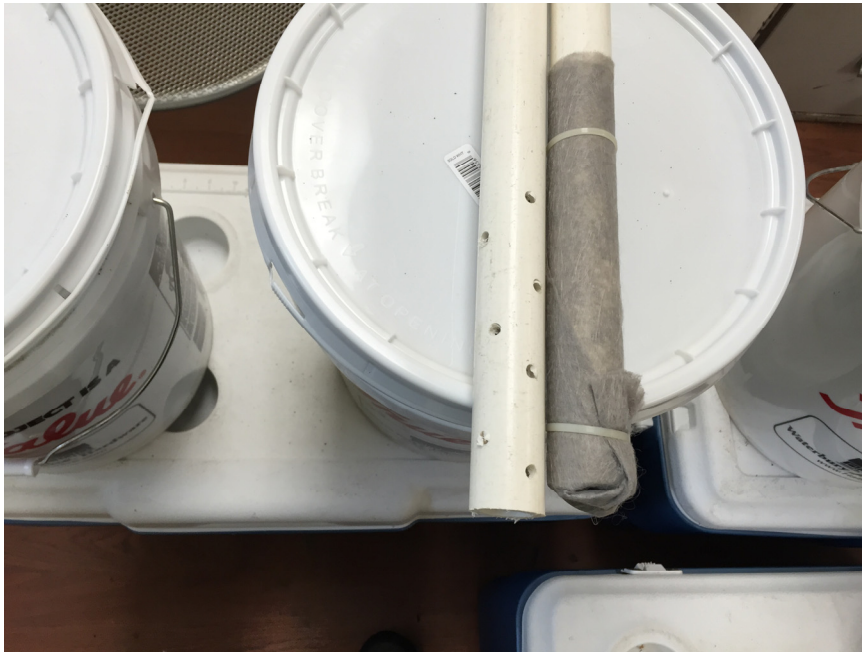
Figure 1. Perforated sample collected tube installed in each bucket
