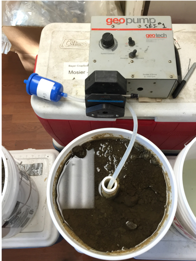
Figure 2. Bucket with saturated WTR and sampling apparatus
